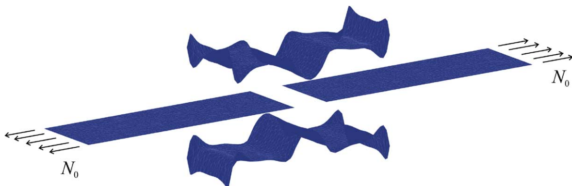
Fig. 15. Scaled deformation of the bonded double-lap joint at the last load step.
